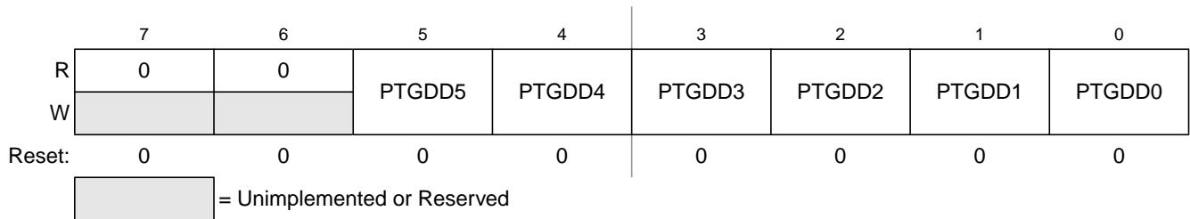
Figure 6-43. Port G Data Direction Register (PTGDD)
